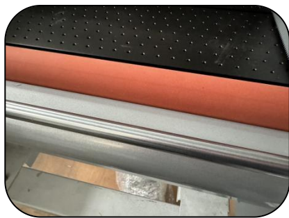
Integrated upper and lower rollers for film laminating
